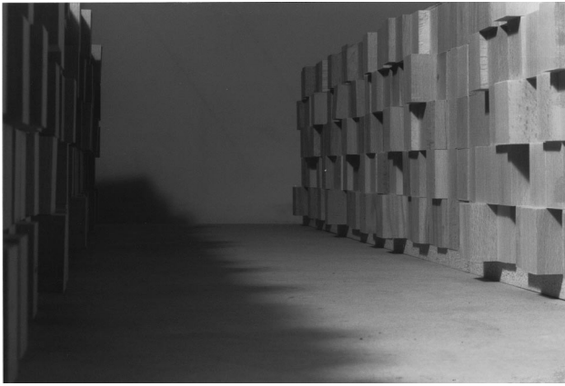
FIG. 3. A \frac{1}{50} scale model of a street. Irregularities of building façades are simulated by an arrangement of wooden cubes. This disposition allows us to reproduce statistically a real distribution of balconies, windows, etc. Details of the experiment will be published in a future paper.
